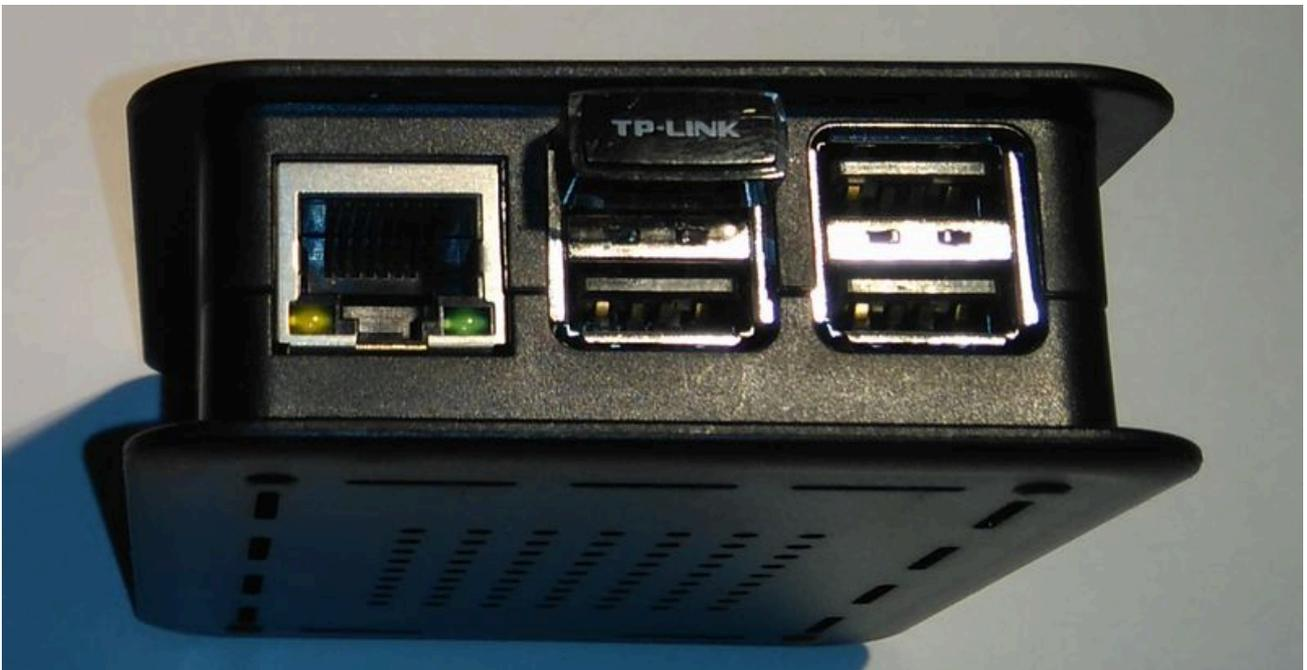
In the picture a Raspberry Pi 3 is shown. Newer ones are equipped with blue USB3.0 sockets. You must connect to the blue socket that is close to the mainboard.
